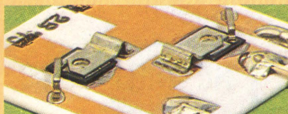
Back-to-back SCR's are superior to triacs in many applications.
